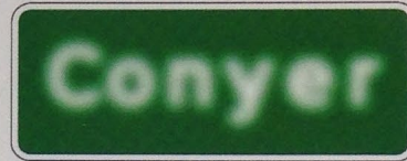
↑ Figure 8.6. Halation and the typeface ClearviewHwy. Not all signs benefit from a bold weight. Backlit and retroreflective signs tend to make type of a heavy weight bleed out by creating an overglow effect on the surface. A simulation of halation showing the effects of overglow on the typeface FHWA (previously applied on highway signs) vs. the typeface Clearview by Terminal Design and Meeker & Associates.
