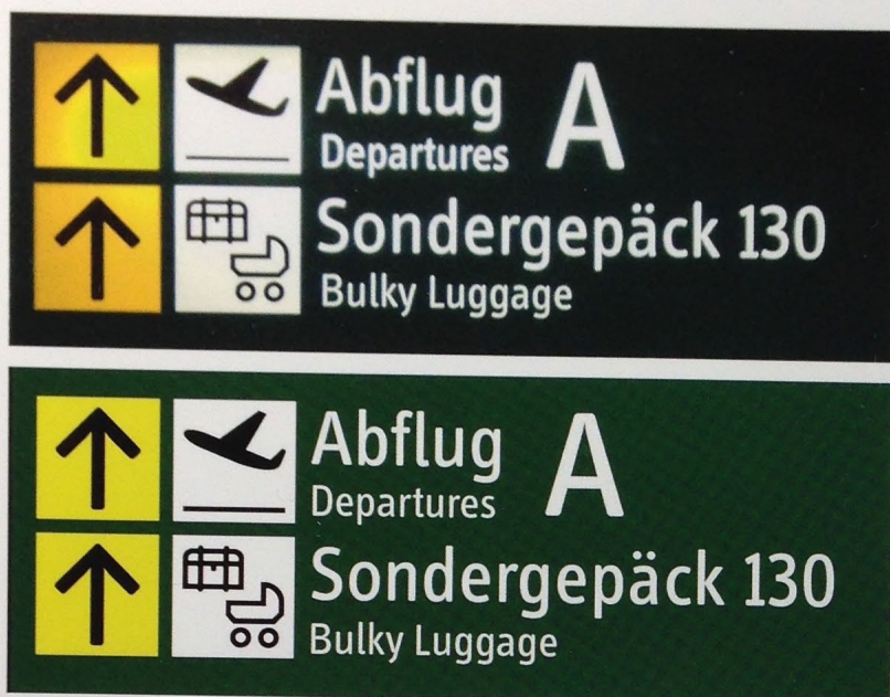
← Figure 8.2. Round corners on FF InfoDisplay. Erik Spiekermann and Ole Schäfer kept the corners of the typeface FF Info rounded, as they found that this feature on backlit signage prevents light shatter and makes it easier to create an even appearance. It also saves considerable time when plotting characters because the blade on the cutter does not have to be lifted and turned 90 degrees but can continue to cut in one line. Illustrated with a photo of a sign from Düsseldorf Airport (top) and a digital rendering (bottom).
